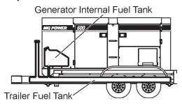
Figure 31 Double Fuel Tank System
